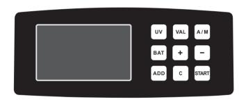
**UV** Turn on/off UV(Ultraviolet) counterfeit detection.
